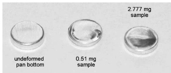
Fig. 6. Photograph of the bottoms of a new aluminum DSC pan (left) and the 0.51 and 2.777 mg samples after completion of the runs in Figs. 1 and 4.
